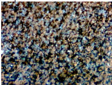
Figure 1 Porous surface of composite metal lapping plate at 200x
