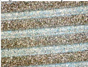
FIGURE 4 PLATE TEXTURE BY MICROGROOVING (FACING) AT 50X
