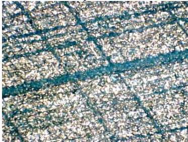
FIGURE 3 “RANDOM GROOVE” PLATE TEXTURE BY 60/80 GRIT DIAMOND PLATED CONDITIONING RING AT 50X MAGNIFICATION
